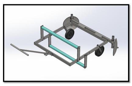
1. Handle 2. Hitching Unit, 3. Mulch Laying Unit, 4. Main Frame, 5. Press Wheel, 6. Earthing Unit
